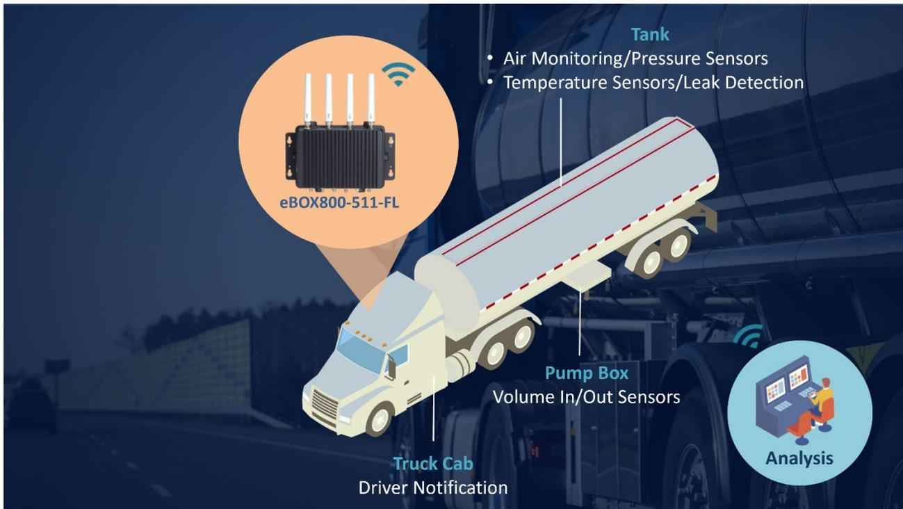
One of the key strengths of the eBOX800-511-FL is its ability to monitor a spectrum of critical parameters promptly. Through the wireless connectivity options of 3G/4G LTE, it ensures the real-time transmission of data from sensors, capturing essential metrics such as fuel level, temperature, pressure, and potential leaks. Real-time monitoring offers a proactive approach to safety and operational efficiency for refueling other working heavy-duty vehicles.
