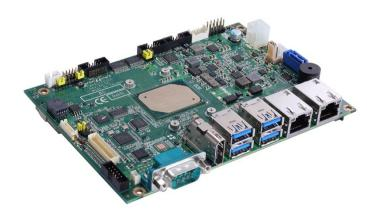
The low power embedded board provides rich I/O including two USB 2.0 and four USB 3.0; there are two LAN ports and four COM ports, with two RS-232/422/485 and two RS-232. The display interface consists of one HDMI and one LVDS, while VGA and eDP are optional. In addition, it features two PCI Express Mini Card slots for various peripheral modules such as Wi-Fi, 3G, and 4G LTE.
