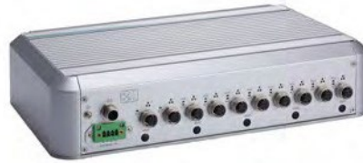
Figure 4. The Axiomtek tBOX400-510-FL is an embedded box PC with an integrated Layer 2 Managed power-over-Ethernet (PoE) switch and countless road, rail, and marine certifications. These allow the platform to be deployed with Genetec software as an onboard video surveillance and analytics platform (Source: Axiomtek).
